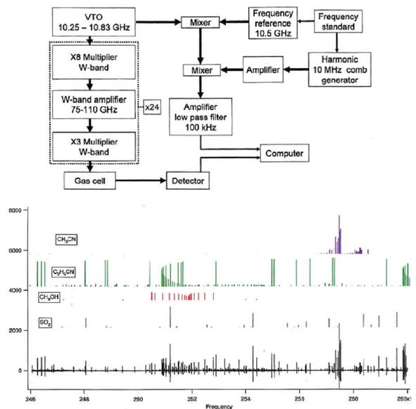
**Fig. 10.** (Above) A solid-state implementation of the FASST technique. (Below) Spectra of four a gas mixture for which partial pressures were ~2 mmTorr (after [34]).
