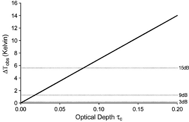
**Fig. 3. The receiver sensitivity and absorbing medium's optical depth variation.**
