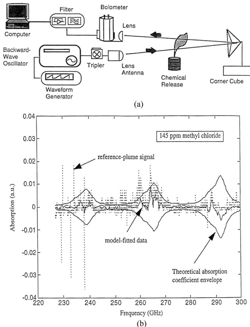
**Fig. 7. (Above) Experimental 215–315 GHz spectrometer in open path measurement sit-up (after [5]). (Below) Absorption of trace methyl chloride in ambient conditions. The difference signal between the reference and the plume (the dotted line), model-fitted signal (the solid line) and the absorption coefficient envelope (solid line) is shown (after [6]).**
