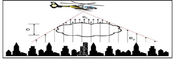
**Fig. 2. A passive airborne radiometer receives radiation from chemical cloud of thickness  $D$  according to BL Law.**
